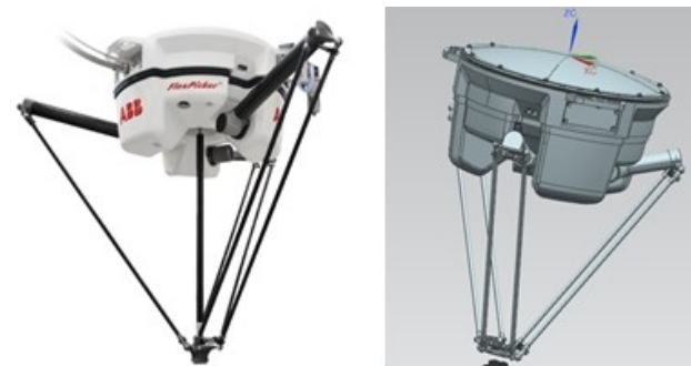
Figure 4: ABB Flexpicker and 3D model
