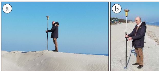
Figure 4. GNSS survey of validations points: (a) on the top of the dunes, (b) on the beach.
