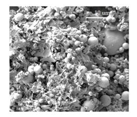
Figure 1. SEM image of the genuine fly ash.
