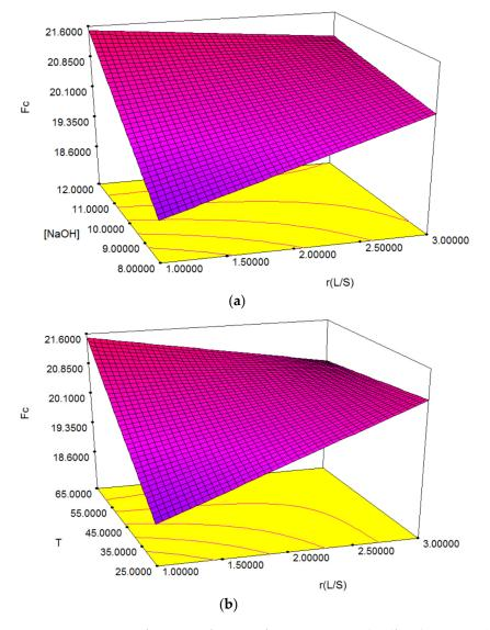
**Figure 7.** Response surface Fc as a function of parameters Xi and Xj (for Xk = constant): (a) Fc = f(X1, X2); (b) Fc = f(X1, X3).
