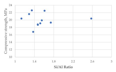
**Figure 6.** The influence of Si/Al rate in different experimental conditions on the the compressive strength of synthesized materials.
