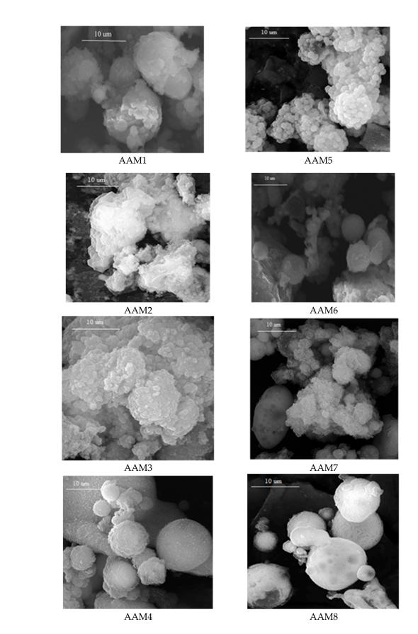
Figure 2. SEM micrograph of the fly ash samples processed by alkali treatments.
