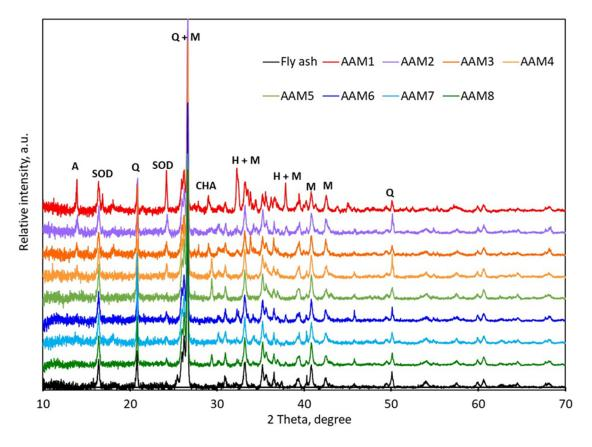
**Figure 3.** XRD patterns for fly ash and selected processed materials (Q—quartz, M—mullite, H—hematite, A—linde type A zeolite, CHA—chabazite, SOD—sodalite).
