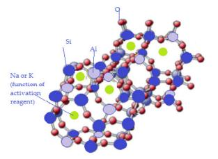
Figure 4. Zeolite precursor formed in the alkali activated process.
