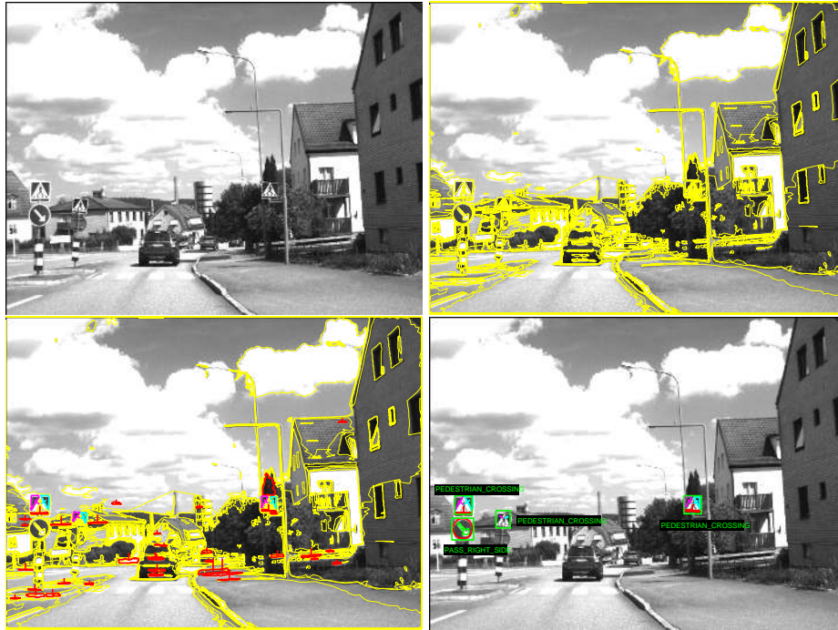
Fig. 3. Upper left: Query image. Upper right: Extracted contours. Lower left: Contours that matched any of the contours in the pedestrian crossing prototype are shown in a non-yellow color. Lower right: The final result after matching against all sign prototypes.
