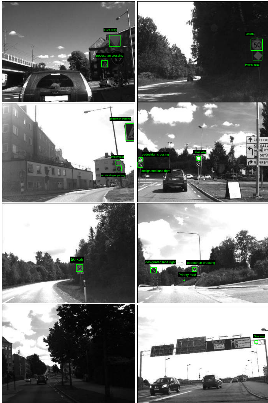
Fig. 6. The first three rows show examples of correctly detected signs. Bottom left shows an example of a missed detection and bottom right shows an example of a false positive, classified as a Give way sign.
