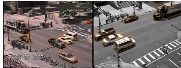
Figure 8. Manually fitted cuboids on vehicles using the calibration parameters.
