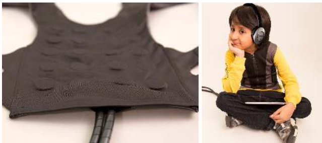
Figure 1: Vest with 20 embedded actuators and story-listening setup
