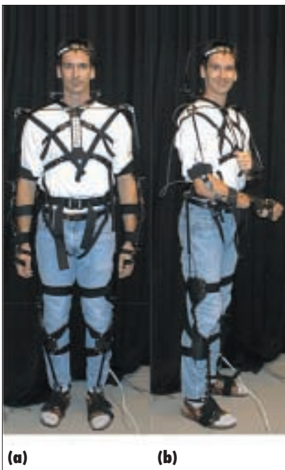
Figure 12. The Sensuit motion-capture system.
