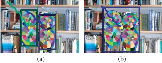
Figure 5. Effect of using gait features. (a) Two targets are properly tracked by using the gait features. (b) Neighboring targets are mistakenly tracked as one target without the use of gait features.
