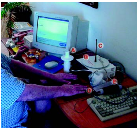
A: Spirometer; B: Home clinical workstation; C: Antenna for ambulatory monitoring; D: ECG plate electrodes; E: Blood pressure cuff.
