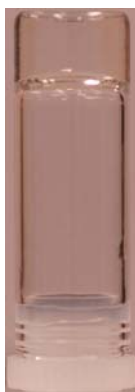
Figure S-1. Optical image of the hydrogel of 2 in water (0.35 wt%, pH = 7.4).
