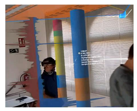
**Figure 10.** MR underground visualization (as seen in the office through the HoloLens HMD) of two boreholes (center and right) and a CPT profile (left). Pointing to the borehole, the properties of the sample are obtained at the given depth. The ground surface can be appreciated at the top (picture courtesy of BGC/Clirio).
