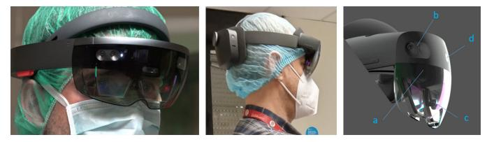
**Figure 3.** Microsoft's HoloLens MR see-through holographic HMD. (**Left**) HoloLens 1. (**Center**) HoloLens 2. (**Right**) detail of some built-in sensors: (a) MEMS projector; (b) two visible-light cameras for head tracking; (c) IR camera for eye tracking; (d) depth sensor.
