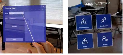
**Figure 4.** (Left) HoloLens 2 Home menu. (Center) The user must tap the desired app/option with their finger, or "air-tap" from distance with the pointer, as in the image in the centre. (**Right**) Main menu of the viewer of the ADA Platform by Clirio.
