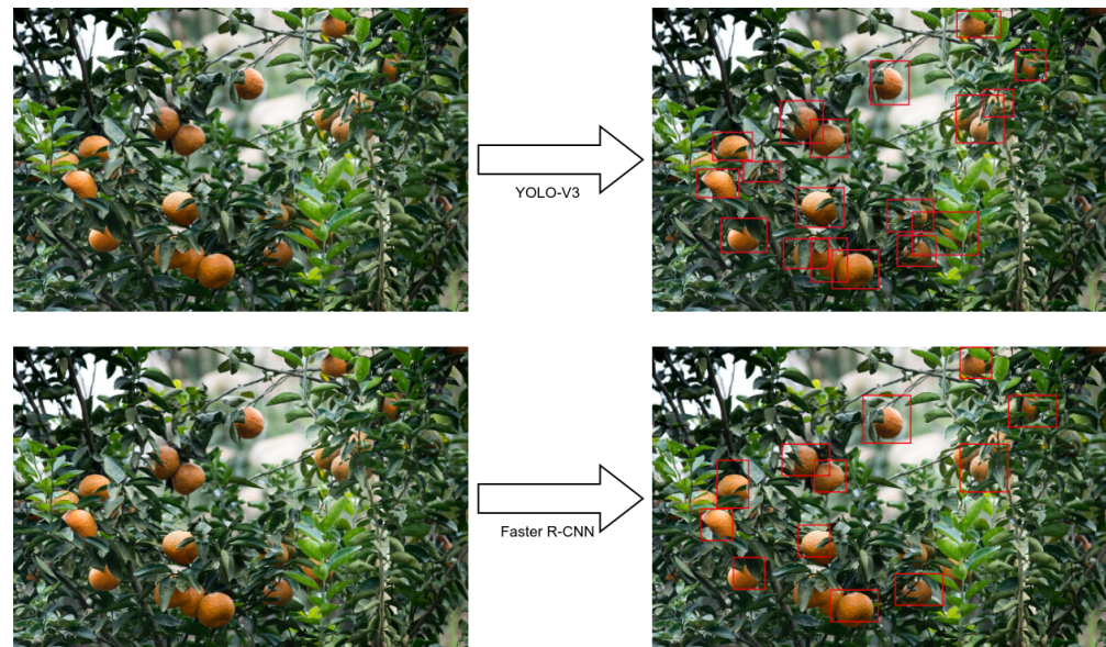
Figure 9. Result of the YOLO-V3 and Faster R-CNN training for this application.
