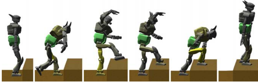
Fig. 4. Stair step planned entirely from scratch.
