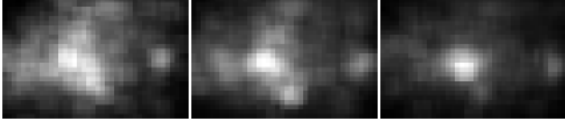
Figure 11: Voting spaces for three neighbouring view-points at a certain scale. Note how strong hypotheses appear at similar locations.
