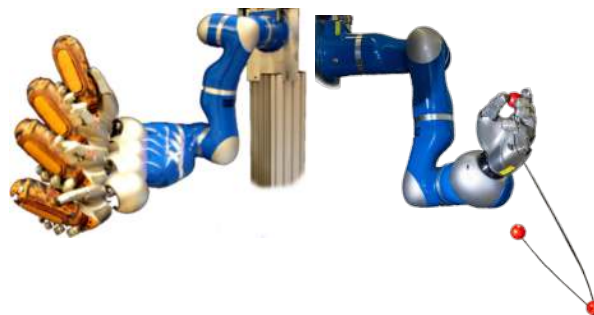
Fig. 1 Two real robot setups that we used for the evaluation of our approach. (left) The KUKA arm playing the maracas musical instrument. We demonstrated a slow version of the rhythmic shaking movement and we progressively increased the speed. (right) The KUKA arm playing with an Astrojax. The robot learned the game from demonstrations.
