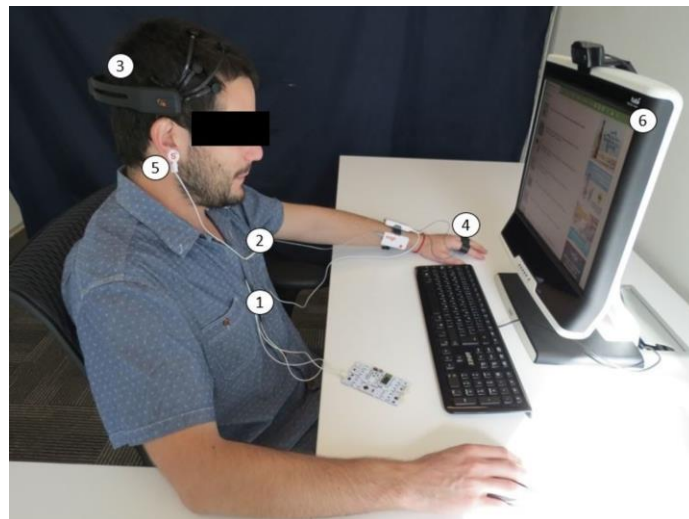
Figure 2. Participant with the sensors runs the experiment. The sensors are: (1) ECG, (2) axillary temperature, (3) EEG, (4) EDA, (5) PPG and (6) eye tracker.
