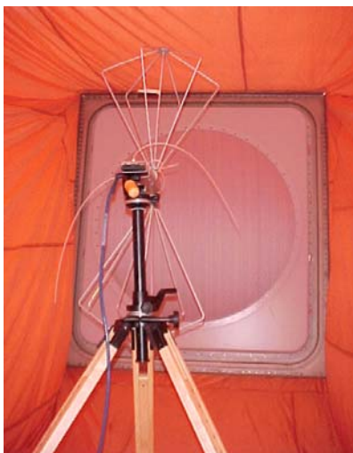
Figure 7: Test set-up: EUT in the VIRC, with an antenna placed in foreground
