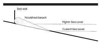
Figure 1. Schematic diagram of response to higher sea level, including a sea wall and a nourished beach.
