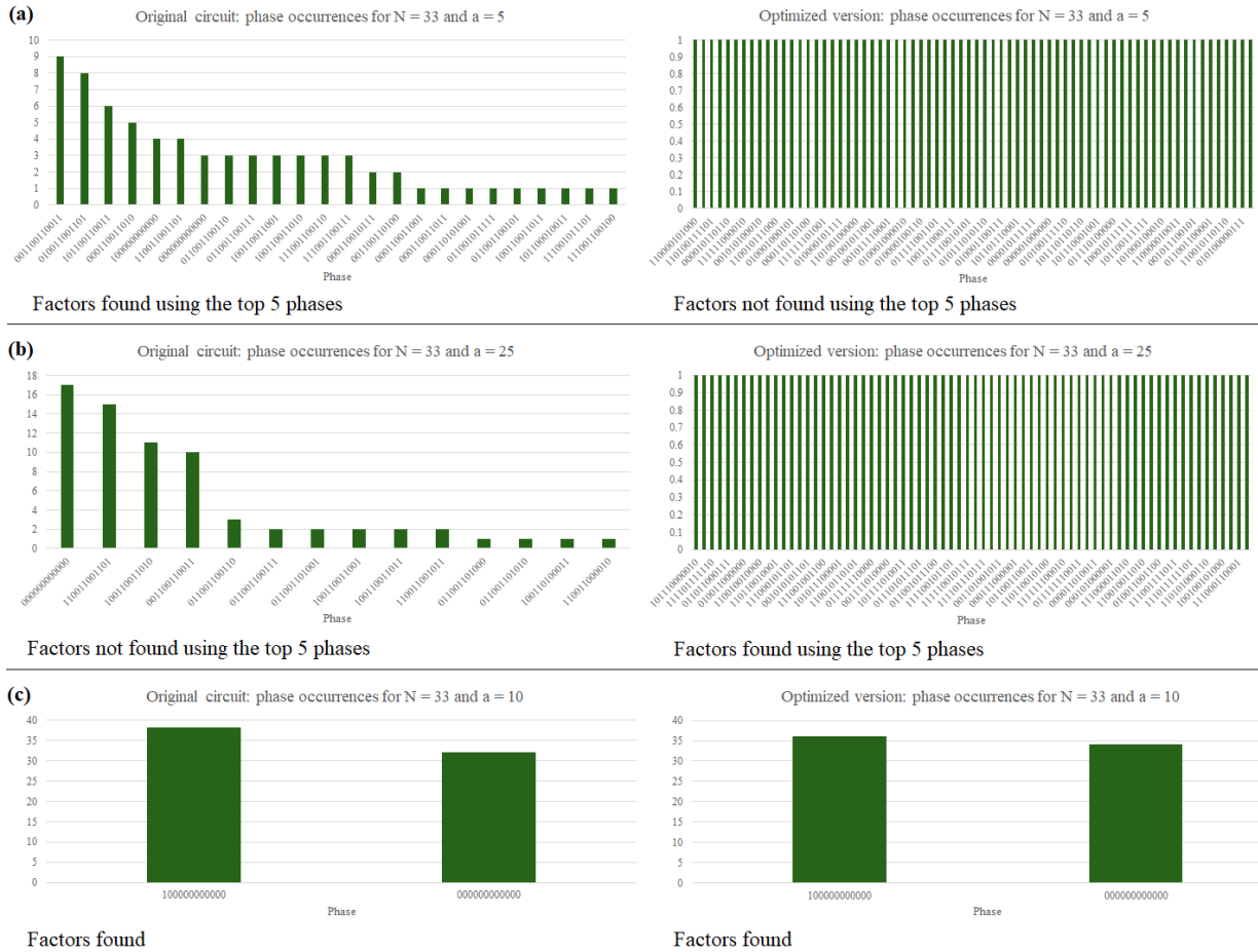
Figure 5: Phase histograms of specific couples ( N, a ) for the original circuit and the optimized version. Phases were sorted according to their occurrences before plotting. (a) illustrates phases found by the two circuits when N = 33 and a = 5 ; the first 5 phases allow factorization only in the original circuit. Differently, histograms represented in (b) consider N = 33 and a = 25 , and entail successful factorization only for the optimized version. Finally, (c) describes very similar phases when N = 33 and a = 10 ; factors are found by both versions of the circuit.
