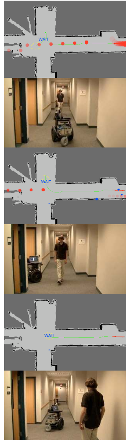
Figure 13. Succession of events of a GSIPP run in ROS. The robot detects a moving obstacle (red circles indicate present and projected path). GSIPP plans a path that avoids it by getting out of the way and waiting for the dynamic obstacle to pass. After the dynamic obstacle has passed, the robot continues its trajectory to the goal.
