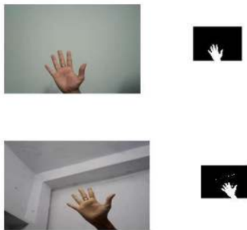
Fig 2.3: image under two different lighting conditions and its output binary image respectively
