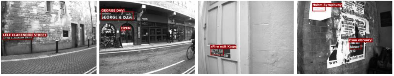
Fig. 5. Examples of wild text found by the robot. The annotations are the raw Tesseract output without any error correction applied.
