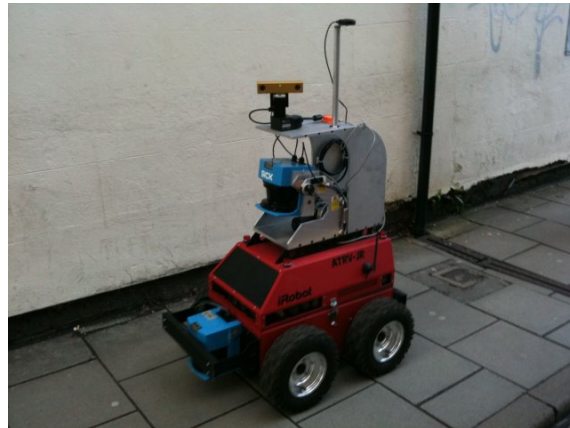
Fig. 2. The data acquisition robot used in this work. Images were captured using the Bumblebee camera mounted on a pan-tilt head.
