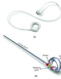
FIGURE 9. The Allergan LAP-BAND ® system (a) and our model (b). The thick part of the band is stiffer than the long part and the two parts are connected by a distance joint.
