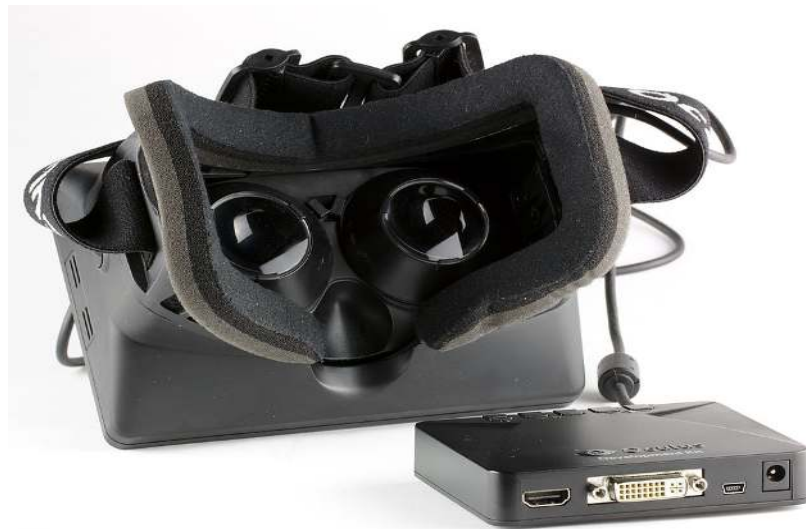
Figure 4. Rear view and control box of the Oculus Rift DK1 virtual reality headset. Adapted from: Stabinger, S. (2013, December). Back and Control Box . Tirol, Austria. Paethon. Copyright 2013, Sebastian Stabinger.
