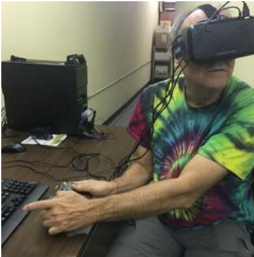
Figure 19. Using the DK3 VR headset and computer set-up. Cords coming off the front of the headset attach to computer hardware. The ability to rotate and move the chair was hindered by these tethers.
