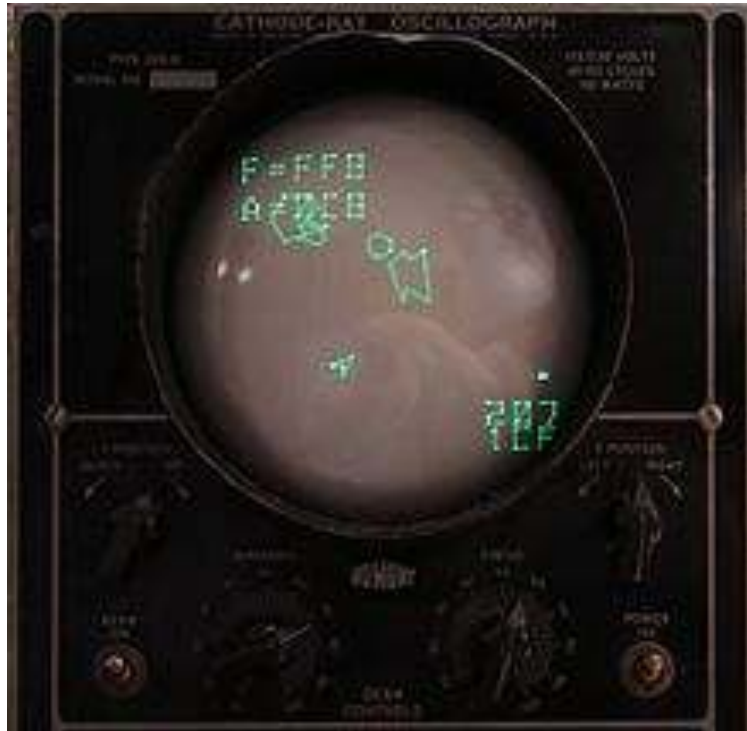
Figure 2. An Asteroids-like video game configured in X-Y mode. Brooklyn, New York, 2013. Adapted from: Hudson, T. (2013, June). Space Rocks (game) . Brooklyn, New York: NYC Resister. Copyright 2013, Trammell Hudson.
