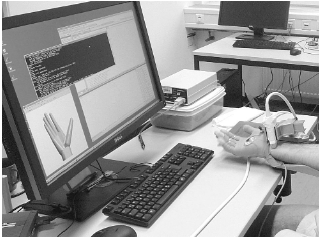
Fig. 3. The experimental setup: the subject would mimic the hand-model movements, as seen on the computer screen; meanwhile, the glove and ultrasound machine would gather hand motions and US images.
