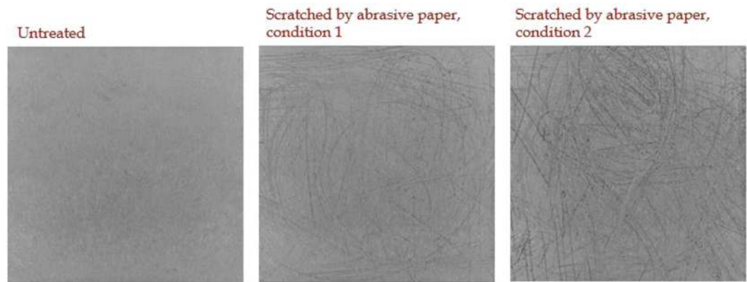
Figure 5. Exemplary sample of LCP Vectra E840i LDS black. The left image shows the untreated surface, the other two images show the platelet's surface scratched by abrasive paper. The intra distance from left to right is: 0.65, 0.35 and 0.23. The mean inter distance is 0.15 \pm 0.01 .
