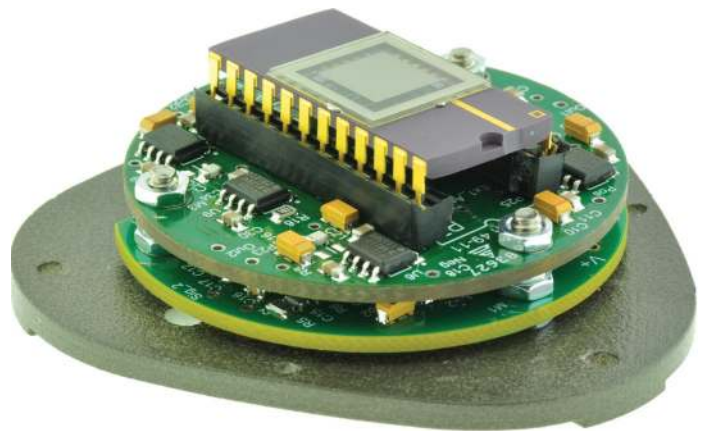
Fig. 1. Photograph of a device used for algorithm demonstration (quadruple mass gyroscope, fabricated in-house without getter material, and mounted on a two stage PCB)
