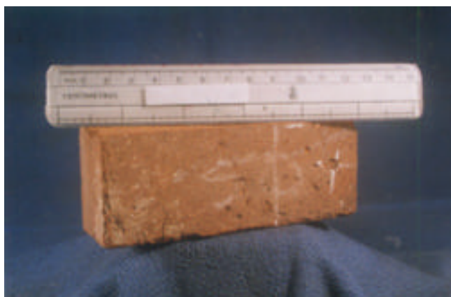
Figure 2. Mixed pond-ash clay bricks obtained on curing at 200–800°C.
