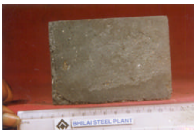
Figure 1. Normal fly ash brick manufactured by using FA, clay and lime binder.
