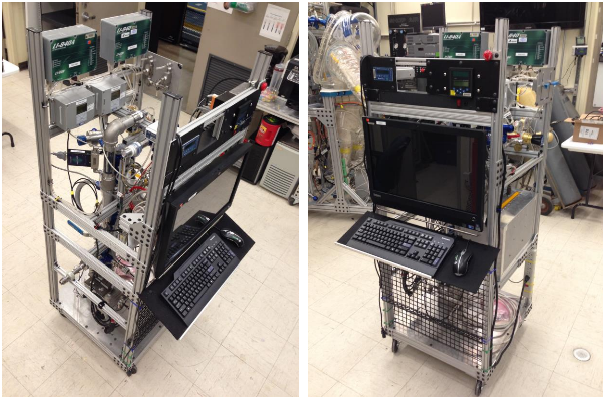
Figure 6. Ventilation Test Loop.
