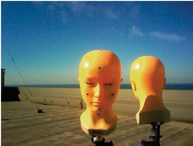
FIG. 1. Observational dummies with built-in UV-B sensors.
