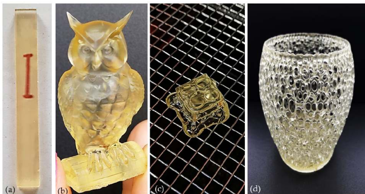
Figure 7. Printed M-AESO-3 resin, transparent bar (a), owl (b), a Lego cube (c), and basket like bowl (d).
