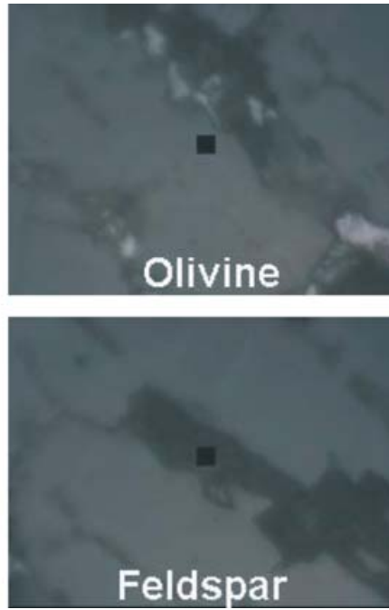
Fig. 3. UV-Vis spectra from a chondrule (barred olivine) from the Allende carbonaceous chondrite. 36\times magnification. The black square is the 4\times 4\ \mu\text{m}^2 aperture through which the spectrum was acquired.
