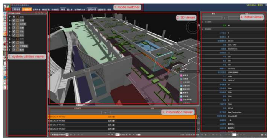
Fig. 6 Five main parts of the system: mode switcher, 3D viewer, information viewer, detail viewer, and system utilities viewer
