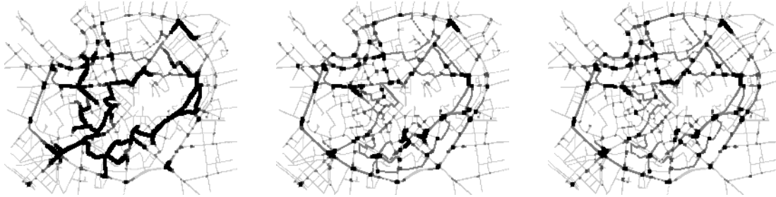
Figure 3. Heat map for the urban scenario when using duarouter, dualterate.py , and VACaMobil (from left to right).
