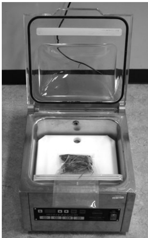
Fig. 1 The MVS35 chamber vacuum-packing machine is shown here with a bag of forage in place ready for vacuum packing
