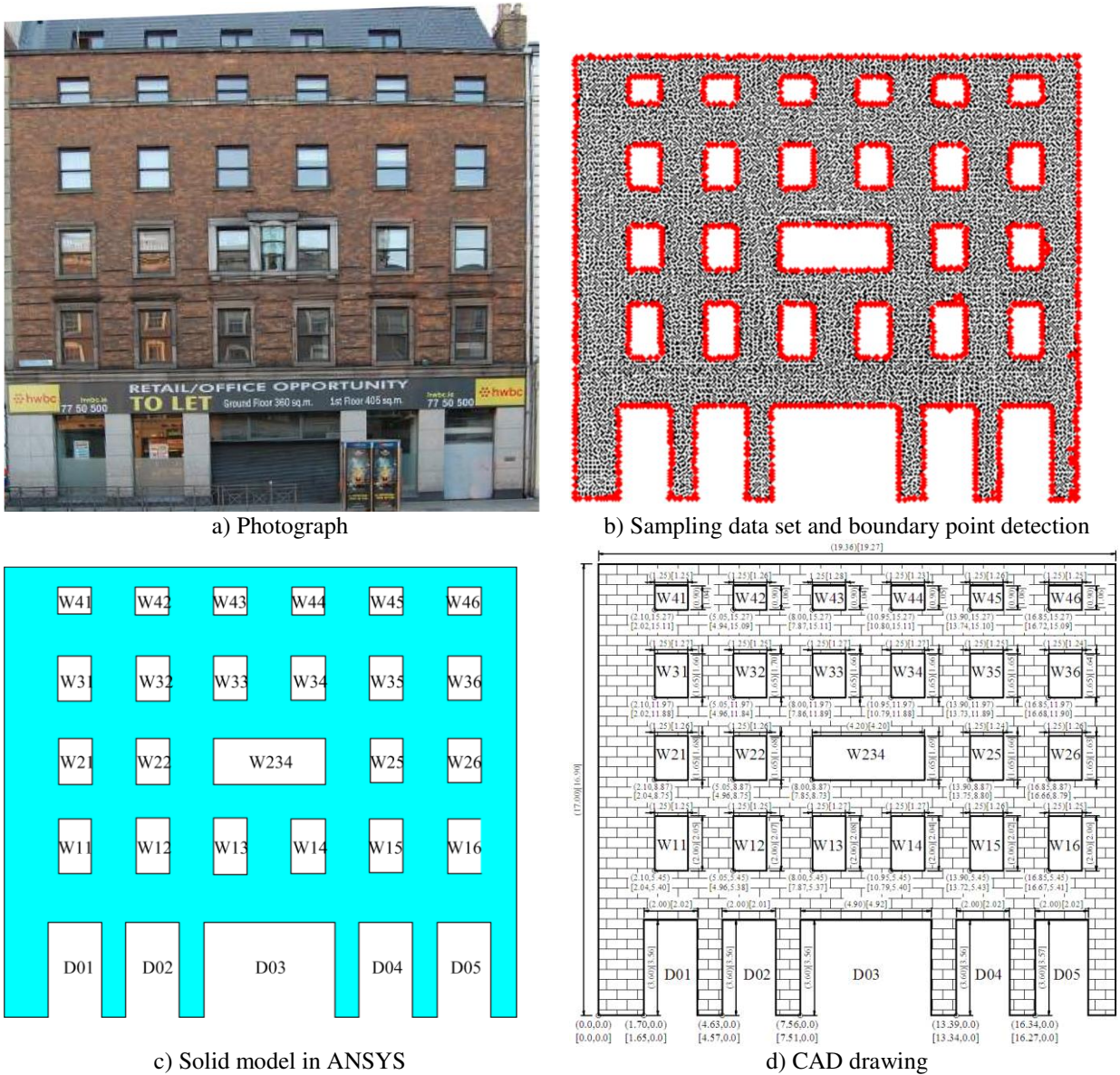
FIG. 5-Post-processing TLS data for Building 3: 2 Westmoreland St. (650,356 points in original set and 35,468 points in re-sampled dataset) (1)
