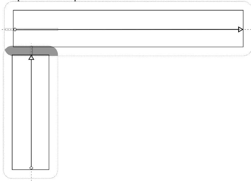
Fig. 2. Graphical depiction of an example wall connectivity intersection operation with two wall “Body” geometries (rectangular); their respective wall “Axis” (a line from square to pointer arrow head); the computed boundary (dotted); boundary intersections (gray); and projections of boundary intersection indicated as narrow rectangle over extended wall “Axis”.
