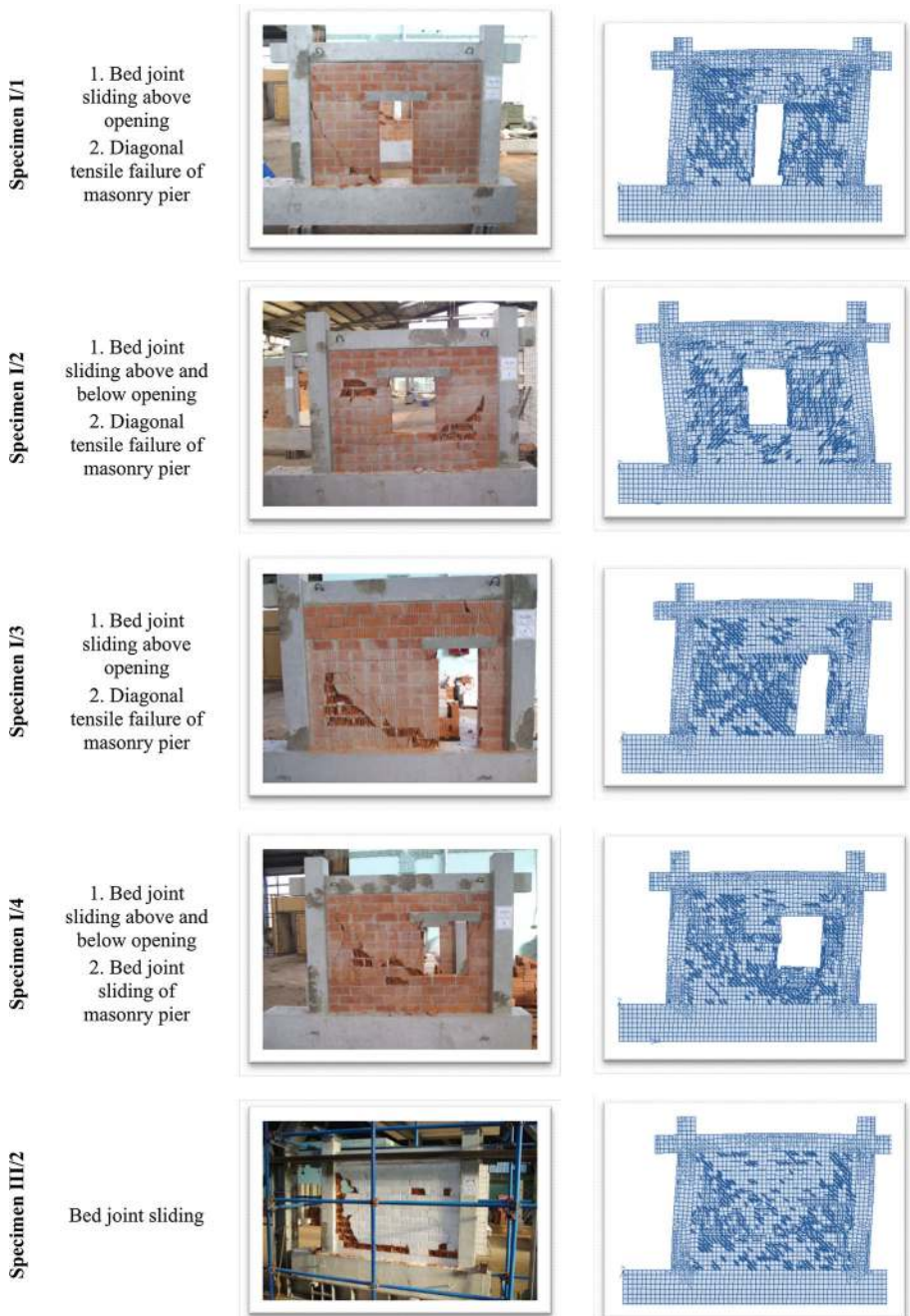
Fig. 7 Calculated and actual failure mechanisms ( crack patterns ) of framed-masonry specimens
