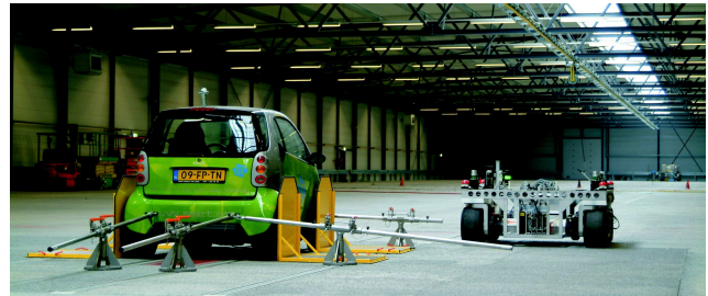
Figure 1: Laboratory setup with intelligent vehicle (left), moving base (right) and chassis dynamometer.
