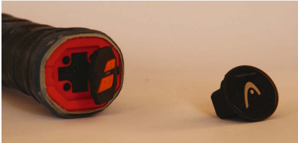
Figure 1. Left side: Handle of a BABOLAT PURE DRIVE PLAY racket with built in sensor. Right side: HEAD TENNIS SENSOR
