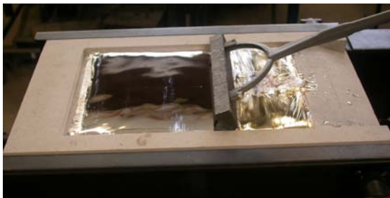
Figure 2: Oxide skim is collected from skimming rig by pulling a blade across the melt surface at regular intervals.
