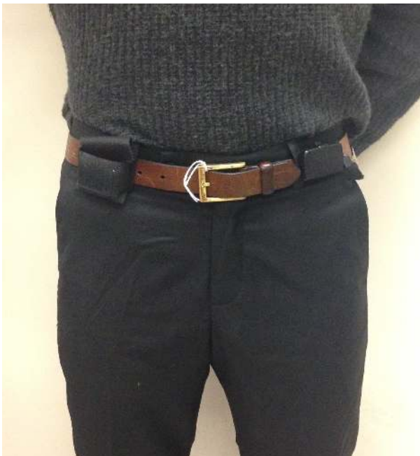
Figure 1. Activity monitor placement with the PiezoRx and the ActiGraph accelerometer positioned on the participants left and right hip respectively.
