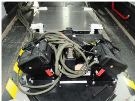
Figure 5: The 3K+ camera system. A low-cost camera system with a higher recording frequency compared to professional photographic camera systems.
