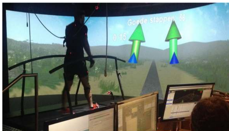
Fig. 1 Virtual reality laboratory equipped with a GRAIL system. The subject receives a target foot progression angle (FPA) through an arrow, which changes color, from red to green, depending on the performed angle
