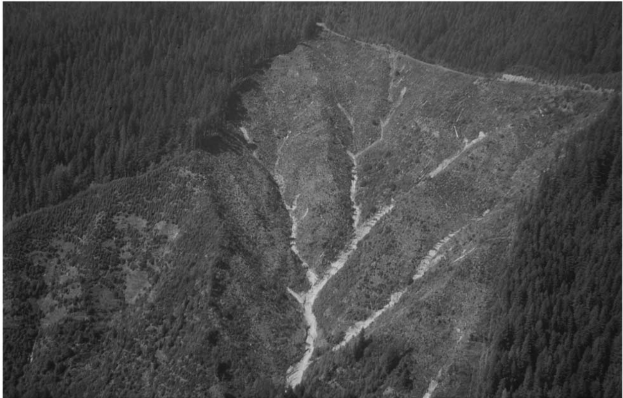
Figure 2. Debris flow valley network in an Oregon Coast Range clear-cut. The combination of elevated water pressure during a 1996 storm and reduced root strength initiated landslides at valley heads that mobilized as debris flows, scouring sediment and Tyee sandstone (white areas) along the runout. Road at top right indicates scale.
