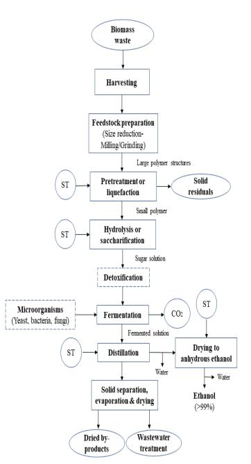
Fig. 1. Flow diagram of bioethanol production from biomass waste (ST: Steam addition) [10, 12, 13].
