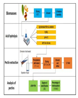
Fig.4. The general process of pectin extraction from biomass waste [52].
