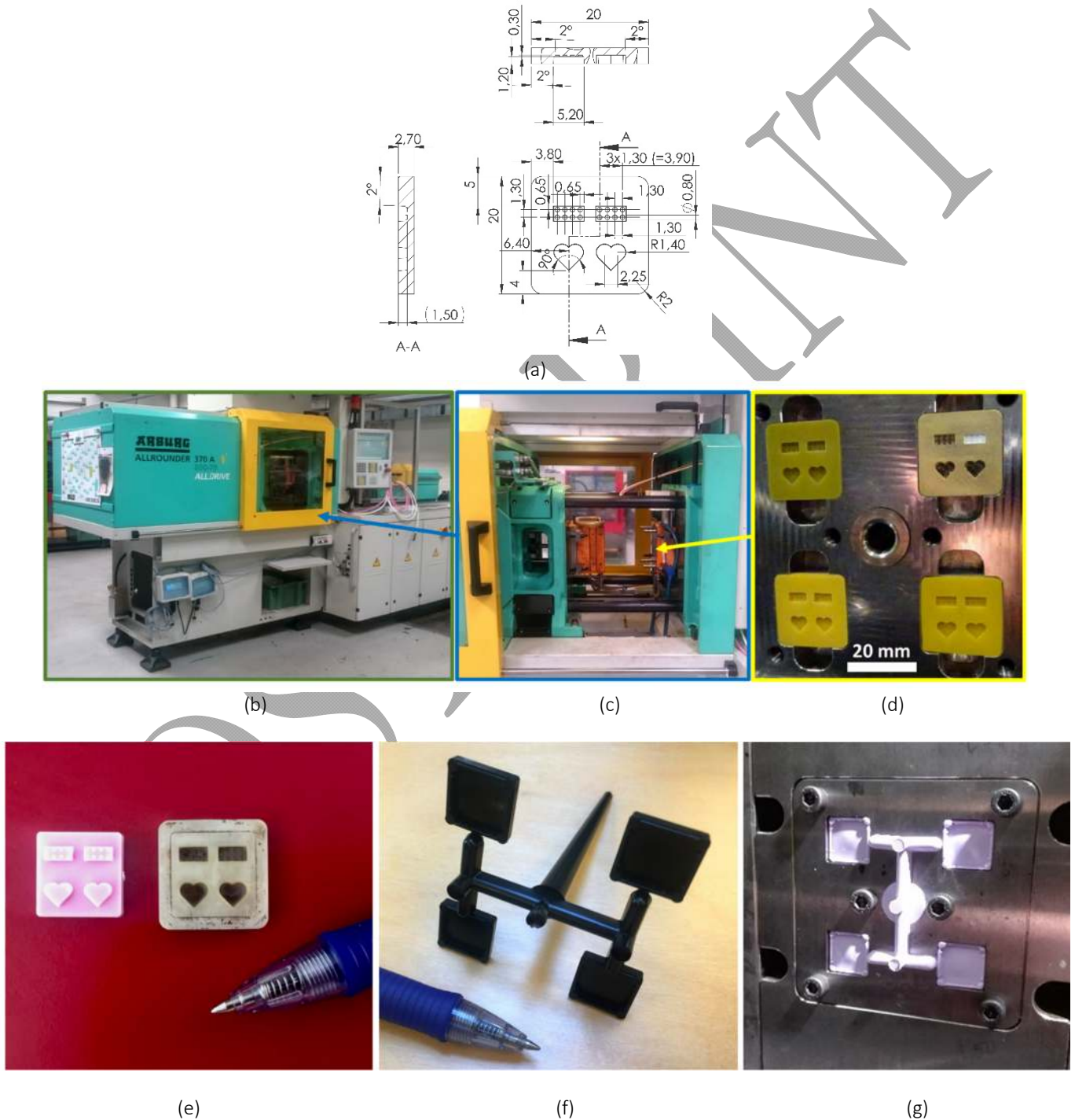
Figure 2. (a) Mould cavity insert considered in this study (adapted from [6]); (b) injection moulding machine; (c) injection moulding tool; (d) four additively manufactured inserts assembled into the moulding tool; (e) plastic part produced by injection moulding (left) using the tool with the additively manufactured insert (right); (f) moulded component produced in each moulding cycle including four part, runners, gates, sprue; (g) complete moulding in the mould before ejection.
