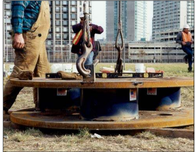
Photo 1.3. – Three O-Cells between two steel plates
