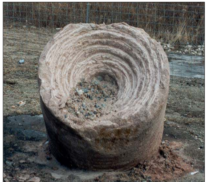
Photo 1.1 - Recovered 1m diameter Core from the “Completely Weathered Rock” zone
