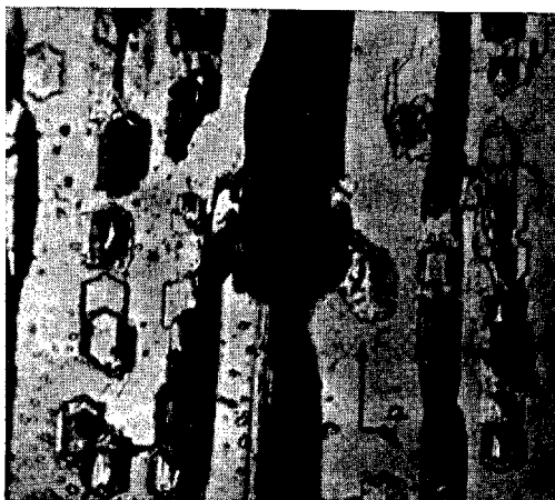
Fig. 5. Different types of etch-pits. 3 C H_2SO_4 , 8 min at 100^\circ C . Refl. light, one Nicol, magn. 230 x. (Phot. Brotzen.)
