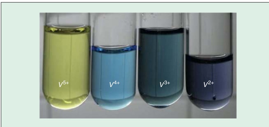
FIGURE 4 – Vanadium exhibits the notable feature of presenting four oxidation states, characterized by different brilliant colors. (Image courtesy of homescience.net; http://woelen.homescience.net/science/index.html .)
